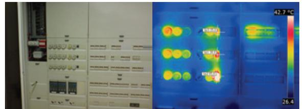
This thermal image shows that the work load during operation is not distributed evenly among the fuse boxes.
