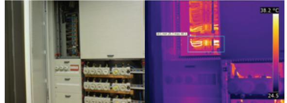
Although these output terminals are definitely hot, the measured temperatures are normal for this kind of load.
