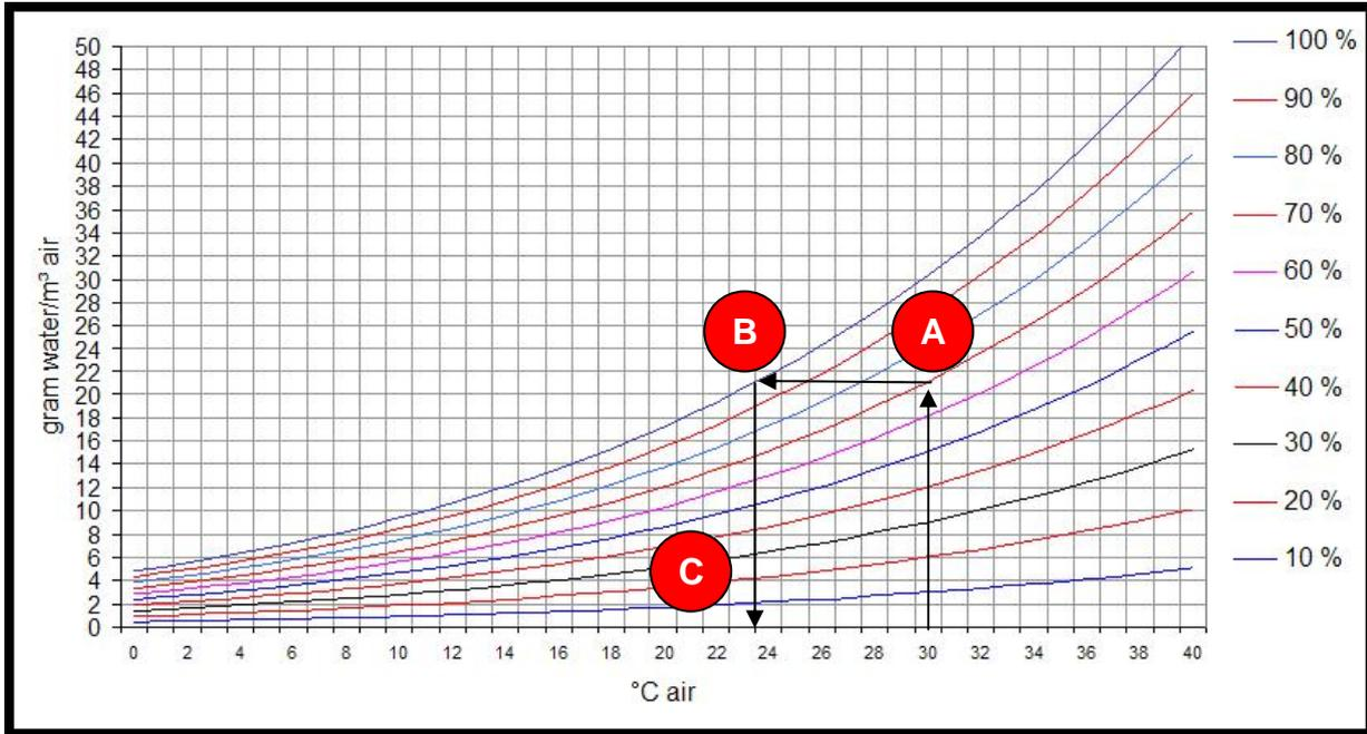
Dew point here is ca. 23,5°C. It means that on any surface below 23,5°C, condensation will occur.
